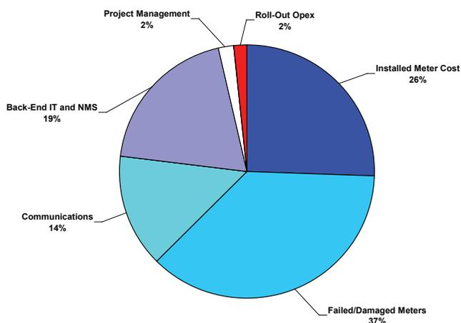
A significant cost involved in a smart metering system in remote communities is the cost of the meters and installation. First, the physical smart meter is more expensive than other electricity meters due to the multitude of functions they can perform.<sup>6</sup> For example, a single phase smart meter with an
